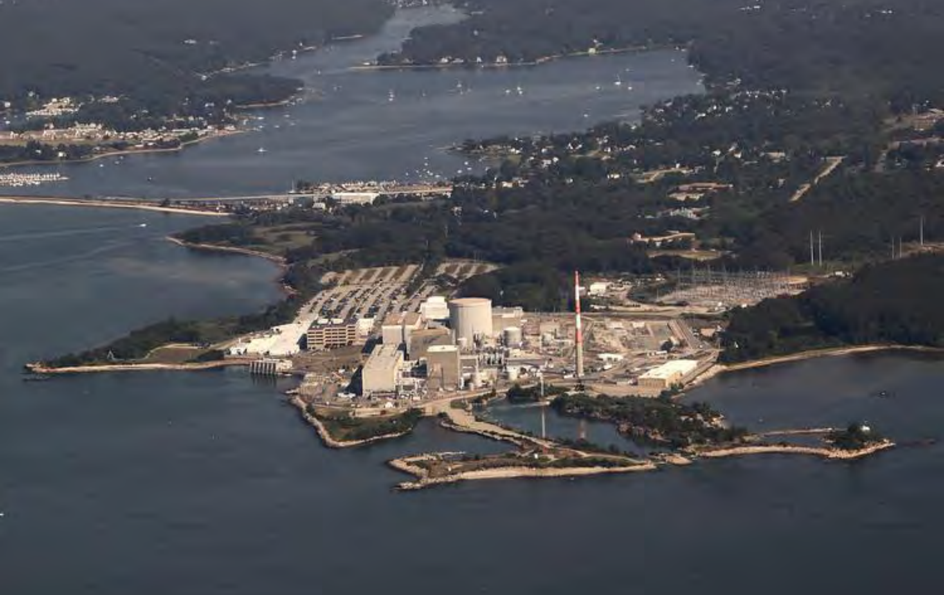
Millstone Nuclear Generating Station, Waterford, CT – 2100 MW Once-through cooling Long Island Sound
